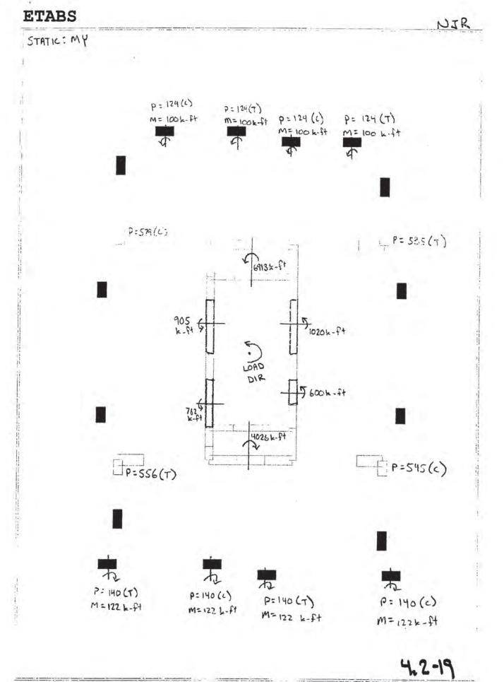
ETABS v8.5.0 - File: 4069-20050509-2.09-CD - May 12,2005 8:42 Plan View - GROUND - Elevation 0 - Kip-ft Units ETABS
