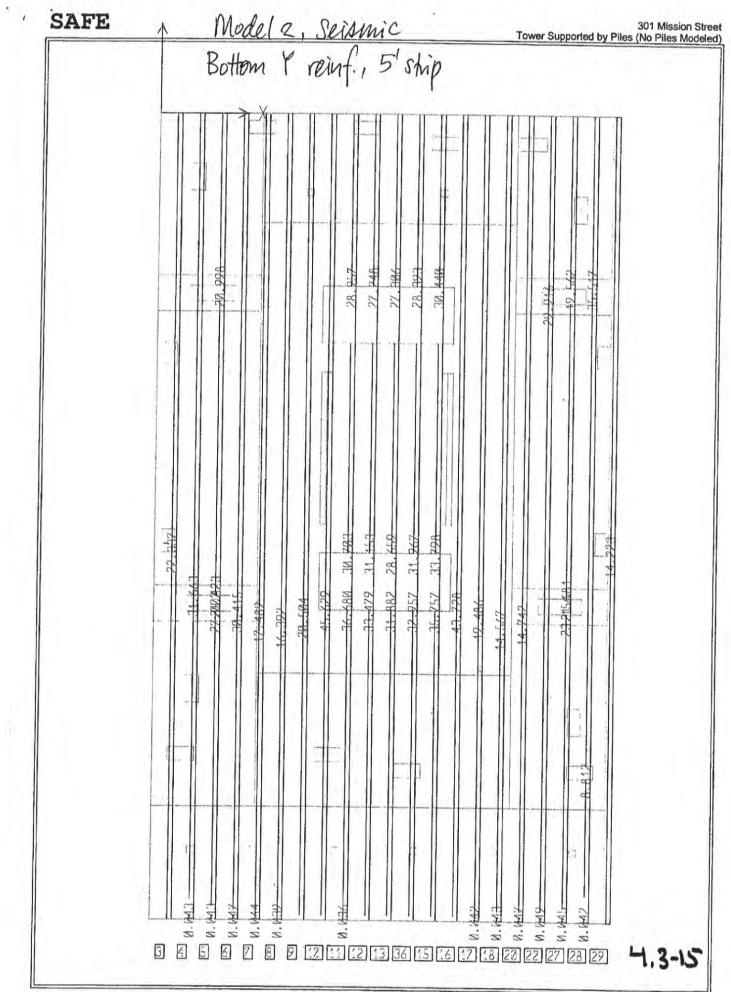
SAFE v8.0.6 - File: 4069-20050523-Tower-Pile-Stiffness-E-strip - May 24,2005 9:41 - Scale: User Scale Bottom Y-Strip Reinforcement (Sq-in) - Kip-ft Units
