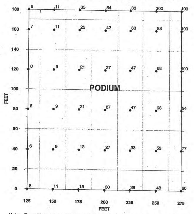
Note: For a 60 foot excavation - Estimated settlement based on foundation pressures provided by DeSimone Consulting Engineers (DCE), dated 17 June 2004 (Podium); Assumes adjacent tower is pile supported and that the soil from a depth of 60 to 90 feet is not compressible and not improved below the Podium footprint.
