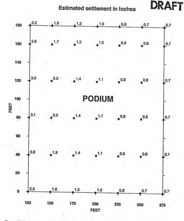
Note: For a 60 foot excavation - Estimated settlement based on foundation pressures provided by DeSimone Consulting Engineers (DCE), dated 17 June 2004 (Podium); Assumes adjacent tower is pile supported and that the soil from a depth of 60 to 90 feet is not compressible and not improved below the Podium footprint.
