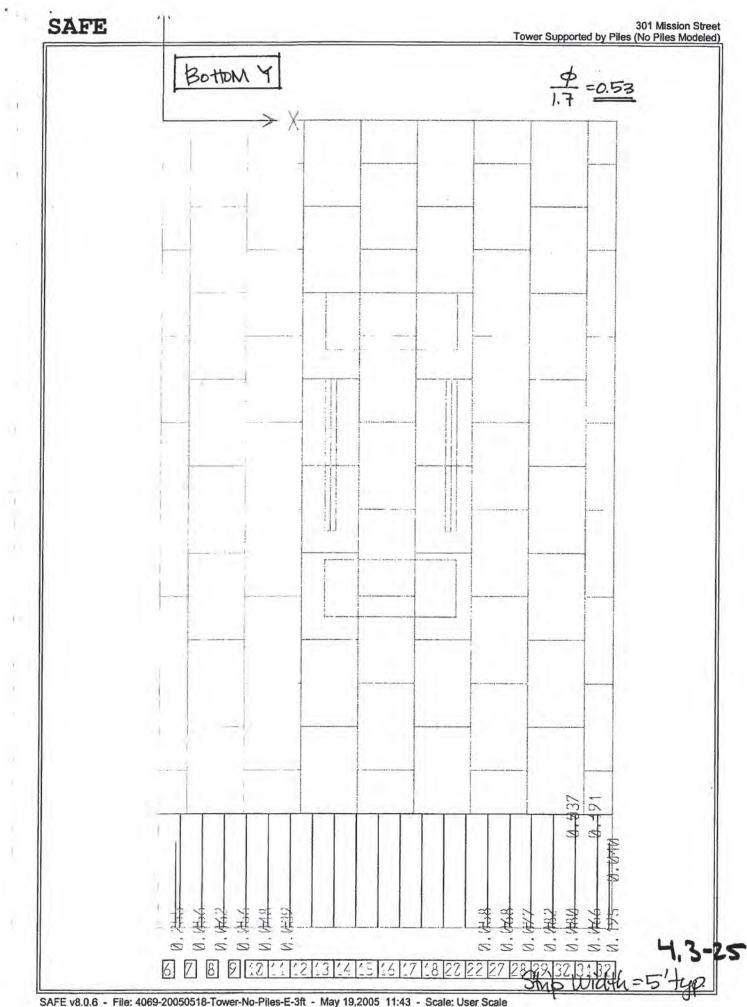
SAFE v8.0.6 - File: 4069-20050518-Tower-No-Piles-E-3ft - May 19,2005 11:43 - Scale: User Scale Bottom Y-Strip Reinforcement (Sq-in) - Kip-ft Units
