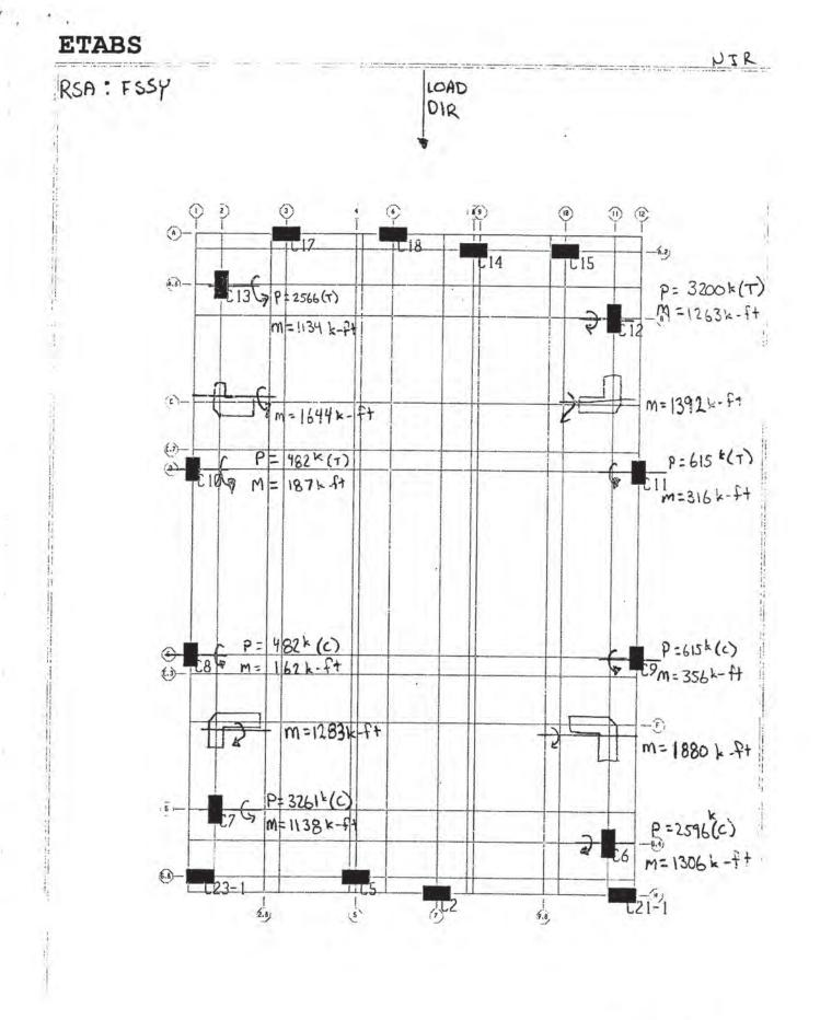
ETABS v8.5.0 ~ File: 4069-20050509-2.09-CD - May 12,2005 7:33 Plan View - GROUND - Elevation 0 - Kip-ft Units 4.2-16
