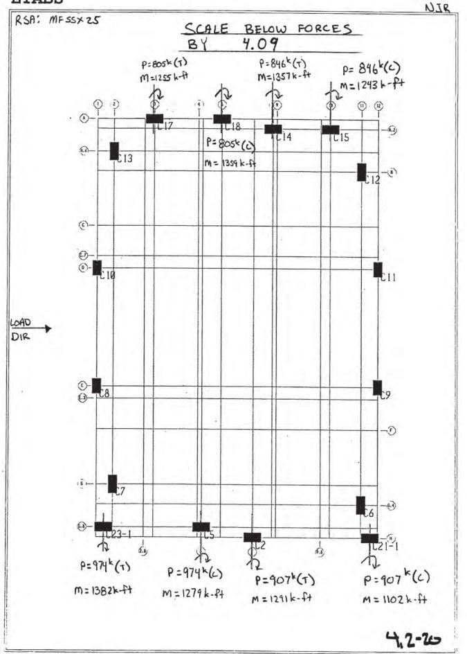
ETABS v8.5.0 - File: 4069-20050509-2.09-CD - May 12,2005 7:33 Plan View - GROUND - Elevation 0 - Kip-ft Units
