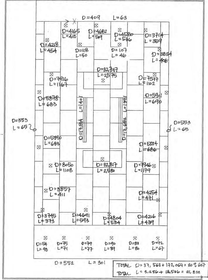
SAFE v8.0.6 - File: 4069-20050518-Tower-No-Piles-E - May 18,2005 17:28 - Scale: User Scale Point Loading (DL) - Kip-in Units
