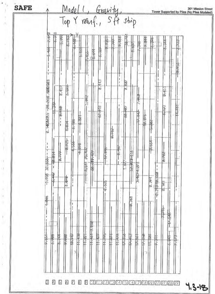
SAFE v8.0.6 - File: 4069-20050523-TR-Stiffness-DL-strip - May 24,2005 9:40 - Scale: User Scale Top Y-Strip Reinforcement (Sq-in) - Kip-ft Units
