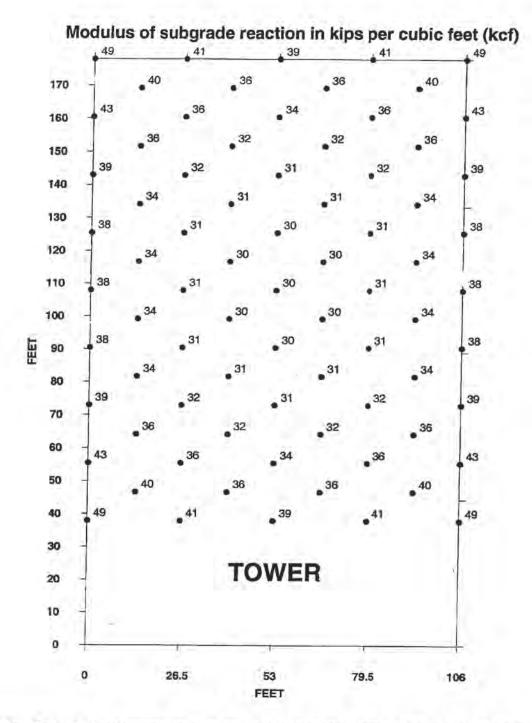
Note: For a 25 foot excavation - Estimated subgrade modulus calculated by taking a uniform building pressure of 14.8 ksf and dividing by the predicted settlement. Assumes Tower is supported by a pile supported mat foundation (106'x140').
