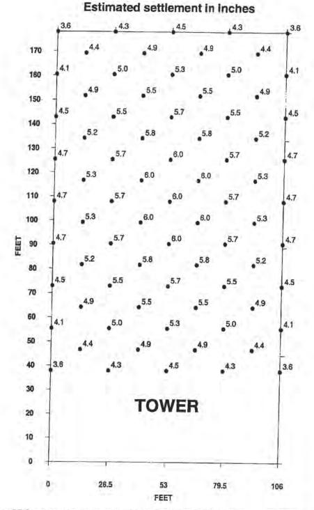
Note: For a 25 foot excavation - Estimated settlement based on a uniform pressure over the Tower footprint (106'x140') of 14.8 kips per square foot (ksf). Assumes Tower is supported by a pile supported mat foundation.
