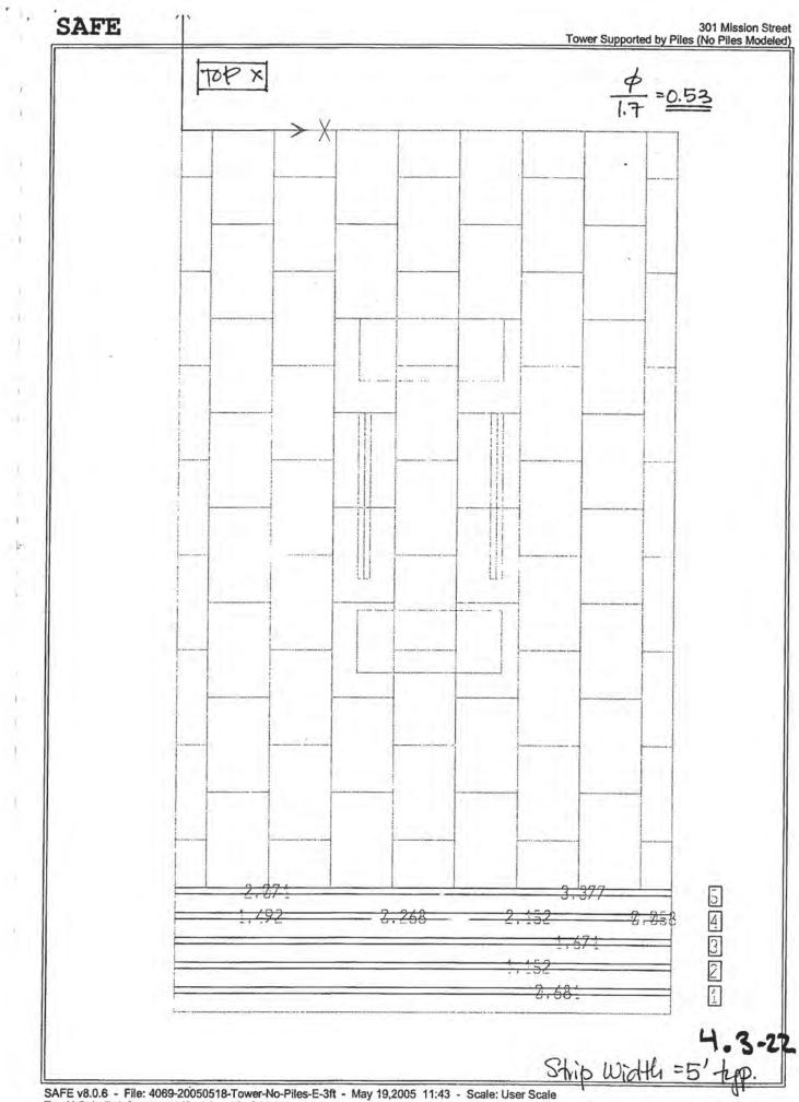
SAFE v8.0.6 - File: 4069-20050518-Tower-No-Piles-E-3ft - May 19,2005 11:43 - Scale: User Scale Top X-Strip Reinforcement (Sq-in) - Kip-ft Units
