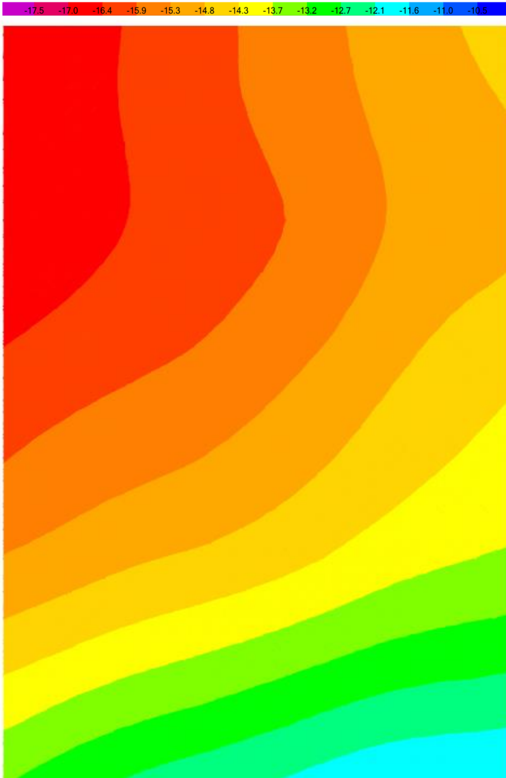
Figure 7-6. Analytical Mat Deflected Shape D + L_{Expected} , kips (Today)
