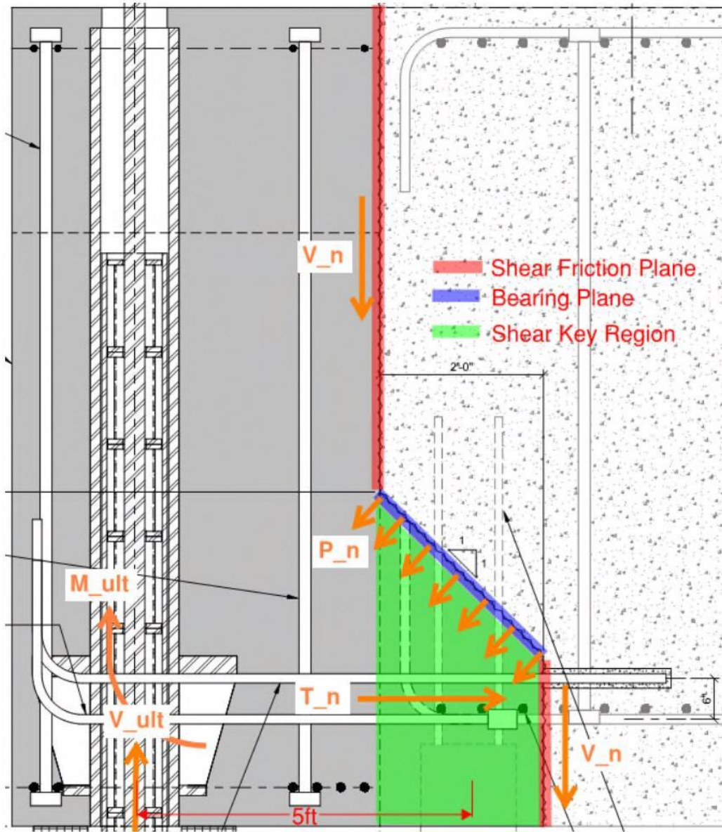
Figure 2. Load path and resisting elements between existing and new pile cap sections.
